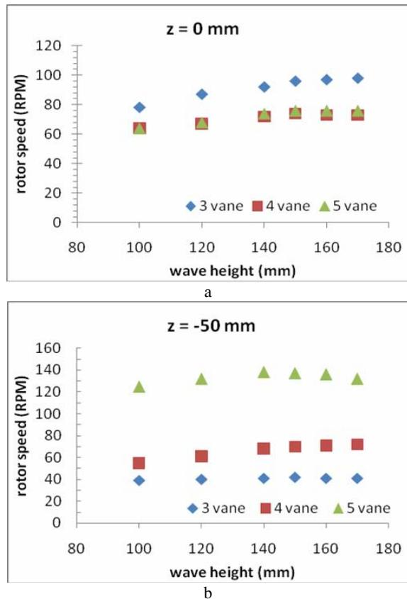
**Figure 5.** Wave height versus RPM; a comparison between 3, 4 & 5 vaned rotors: a.  $z = 0$  mm; b.  $z = -50$  mm.
