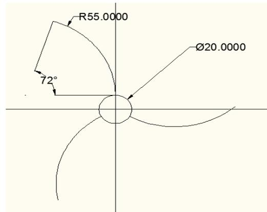
**Figure 3.** Profile of the Savonius rotor vanes.
