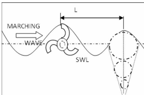
**Figure 1.** The Schematic Representation of a Savonius Rotor utilizing the orbital motion.
