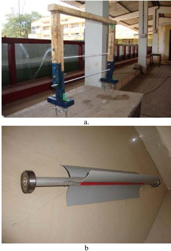
**Figure 2.** The Savonius rotor: a. fixture frame; b. rotor with redstrip fixed on bearings.
