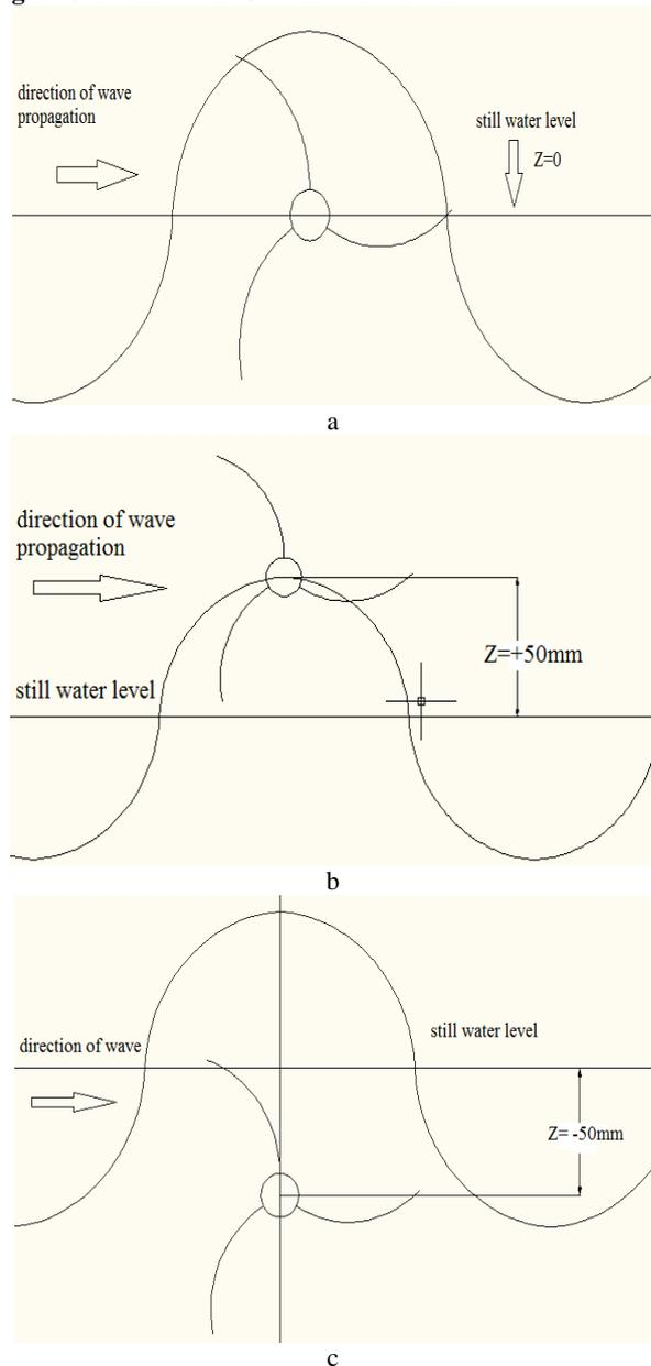
**Figure 4.** Experimental Set-up: a.  $z = 0$  mm; b.  $z = +50$  mm; c.  $z = -50$  mm.
